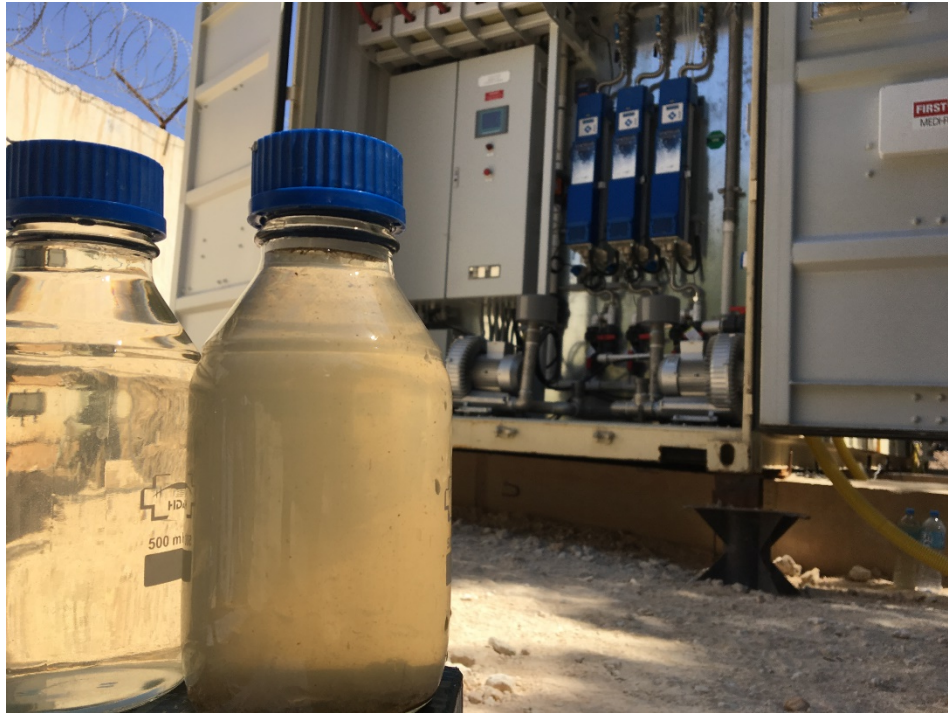
FIGURE 7: REGEN 40 PLUS+ INFLUENT AND EFFLUENT SAMPLES TAKEN 6 WEEKS AFTER STARTUP
